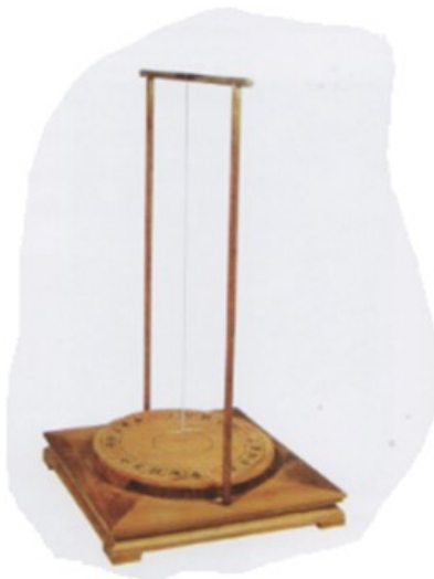
Magnetised needle suspended on a thread
