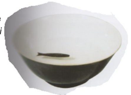
Magnetised needle in bowl of water
